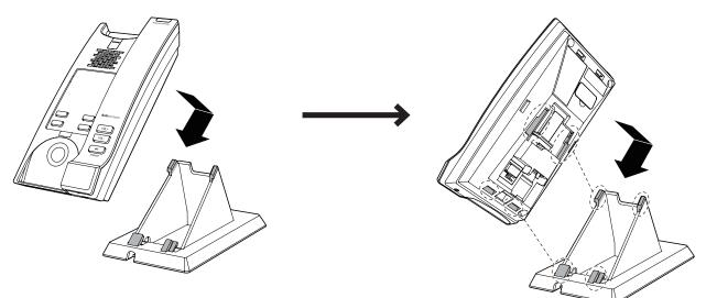
2. Connect both the ethernet cable and coiled handset cord to the telephone base and route them along the wire ducts accordingly. Install the telephone base as shown below.
