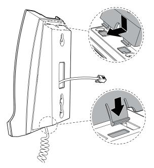
4. Mount the telephone base on the wall by positioning the eyelets on the mounting bracket against the mounting studs. Then, slide the telephone base down on both mounting studs until it locks into place.
