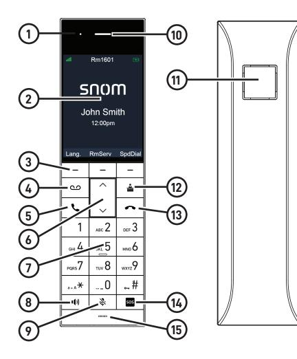
Handset Battery charging light 1 2 Colour screen 3 Soft keys (3) Perform the action indicated by the on-screen labels. **MESSAGES** key 4 **TALK** key 5 6 navigation keys 7 Numeric dial keys I) SPEAKER key 8 **MUTE** key 9 10 Handset earpiece 11 Speakerphone 12 **FRONT DESK** key OFF/Cancel key 13 14 SOS EMERGENCY key 15 Microphone
