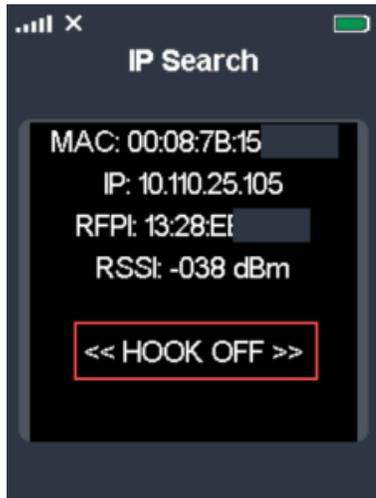
6. Place the next base station where the signal reduction reaches the value of **75dBm**.
